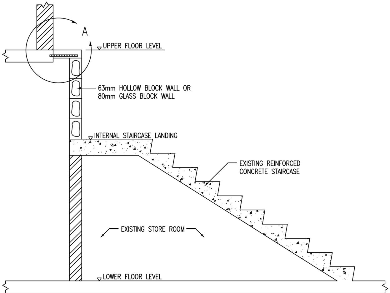
ELEVATION VIEW OF INTERNAL STAIRCASE
