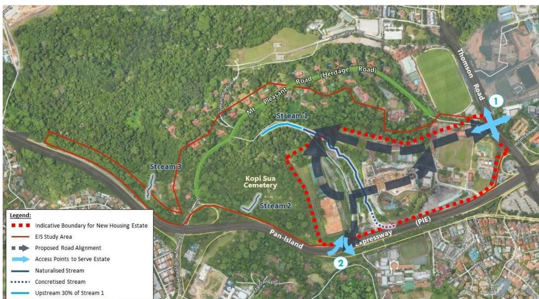
Figure 3: The road network has been revised to take access via the existing Onraet Road off PIE. With this adjustment, two of the three streams (Streams 2 and 3) will be fully retained, and the adjacent Kopi Sua Cemetery will not be affected.
