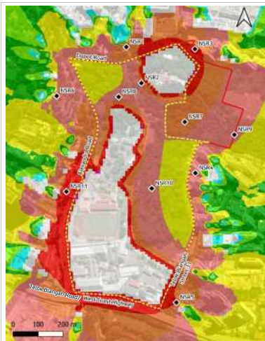
Demolition Works: Unmitigated ( L_{Aeq} 12 hours)
