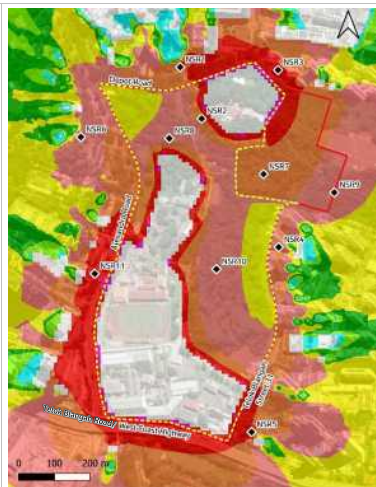
Demolition Works: Unmitigated ( L_{Aeq} 5 minutes)
