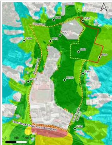
Demolition Works: Mitigated ( L_{Aeq} 5 minutes)
